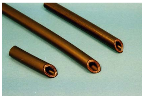
Power steering hoses
